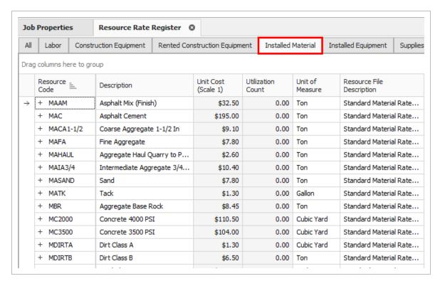
Above is an example of the Installed Material tab in the Library Resource Rate Register.
