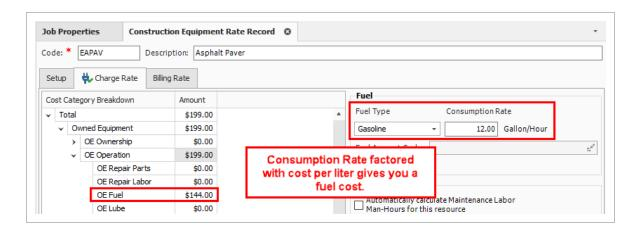
The below figure shows where consumption rates are defined on the Construction Equipment Resource Rate Record.
